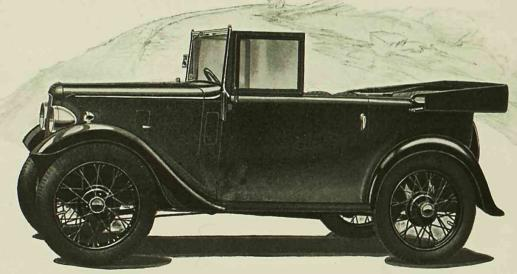
The cars can be finished to choice of Austin colours—upholstered in hard wearing leather cloth. There are direction indicators with automatic return switch, electric windscreen wiper, driving mirror, floor draught excluders, spare wheel and tyre with cover and those accessories shown on chassis specification. Exterior and interior fittings chromium plated. Triplex glass screens.
