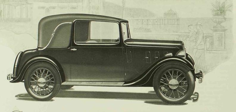
MODERN car of elegant proportions. The front seats are separately adjustable, they tilt forward, and this, with the very wide doors, makes access to the rear seats extremely easy. The spare wheel with cover is carried at the rear of the car. The hood is easily operated and is secured in any of three positions, closed, half-open, fully opened, and is thus adaptable for all weather conditions.
