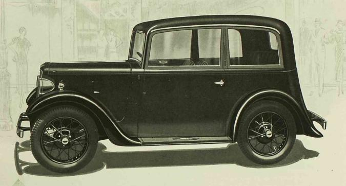
NEW body on modern lines with sloping radiator cowl, longer bonnet with ventilating shutters, new wings and valances, and bumpers. The spare wheel carried under cover at the rear, a Pytchley sliding roof and rear quarter windows that open to assist ventilation—are some of the new features embodied in the latest Seven Saloon de Luxe.
